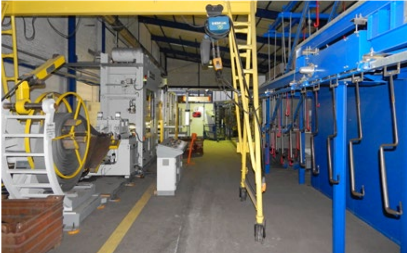
The timed production line: from uncoiling (l.) to powder coating (r.)
